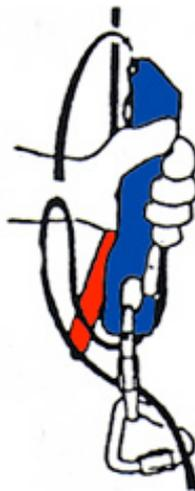
Once the descender is on the rope it is important that it is 'locked off' before you put your weight on it. This also applies when passing obstacles. Locking off is for safety and avoids descent before you are ready. To lock off fold and push the free hanging rope through the oval krab and thread the resulting loop over the top of the descender.
